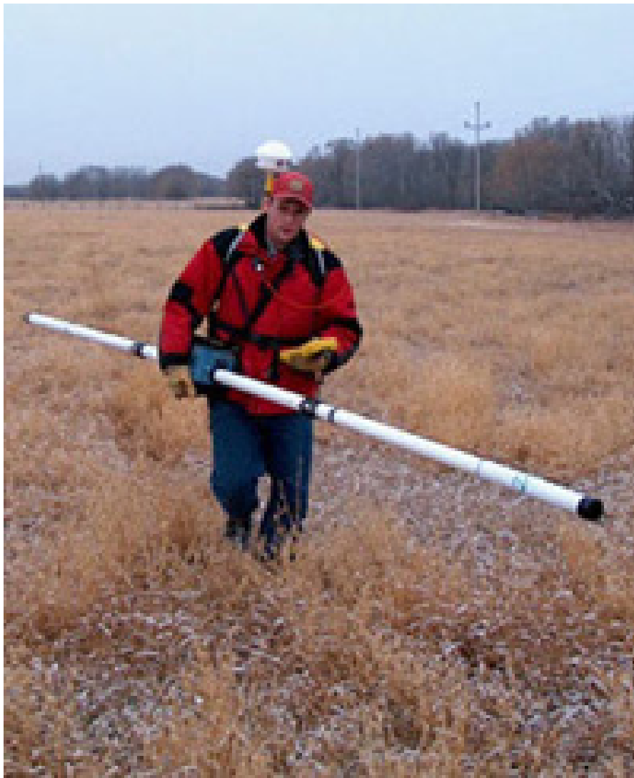
Figure 1 Photo of the EM31-MK2 in Use (Geonics, 2012)
