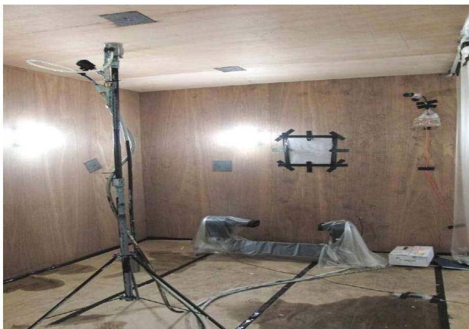
Fig. 3, PDX Atomizer and laser particle analyzer testing
