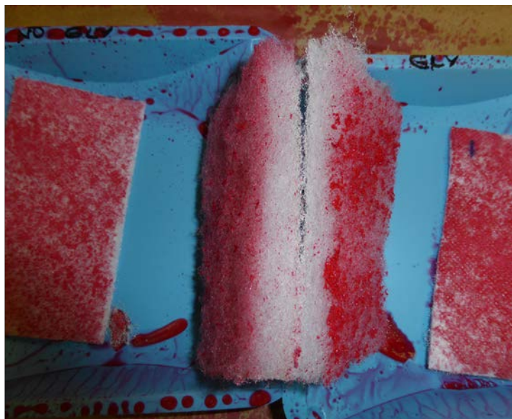
Figure 11. FX2 GF (left) and standard FX2 (right) coating polyester coupons.
