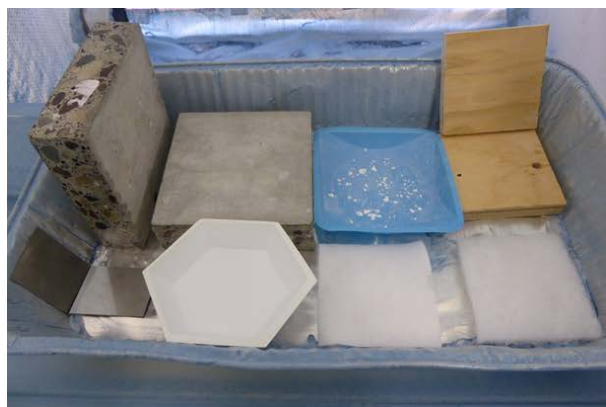
Fig. 10. Fogging Coupon Specimens Before and After Fogging
