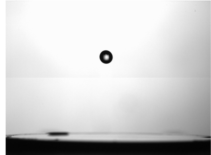
impact of a water drop on a thin-film. Guildenbecher et al, 2013, Exp. Fluids .
