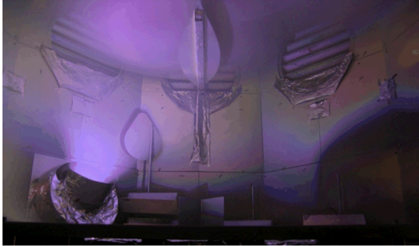
Figure 1. The ion source in operation within the coating chamber.
