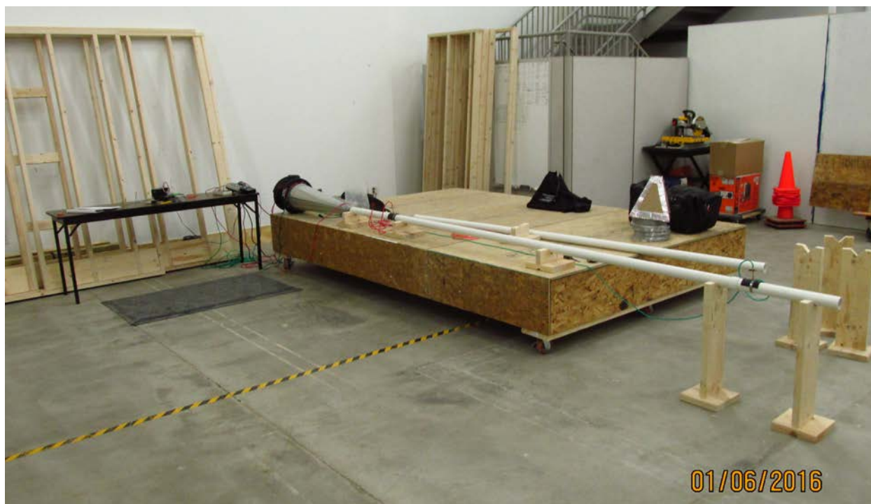
Figure 7. Example test setup with duct blaster connected to a PVC pipe. The conical steel reducer is also shown.
