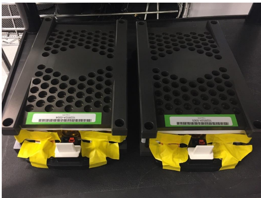
Figure 5 - Photo of two of the prototype 100+ Ah can cells in compression plates for testing. These cells were shipped to Argonne National Laboratory for testing to complete Deliverable 9.2. The yield of this cell prototyping campaign was 100% (8/8 cells good) according to the established program yielding criteria.
