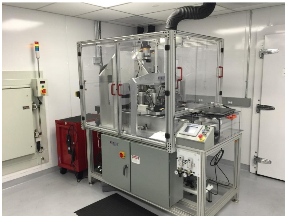
Figure 4. High volume manufacturing method equipment to produce large footprint electrodes.
