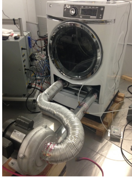
Figure 21. Outboard blower setup required the bottom of the front panel of the HPCD to be cut out.
