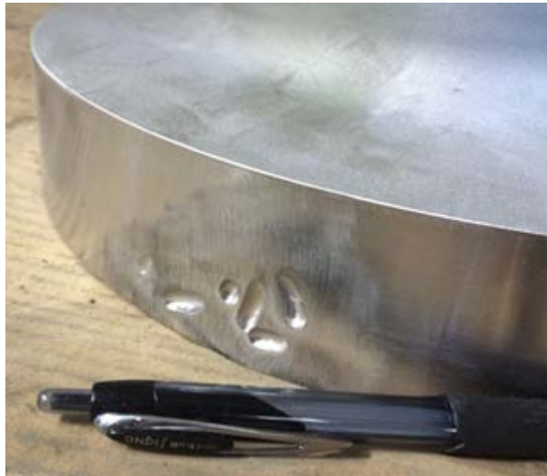
Figure 3-3. Surface Defect in the Exhaust Reducer Housing
