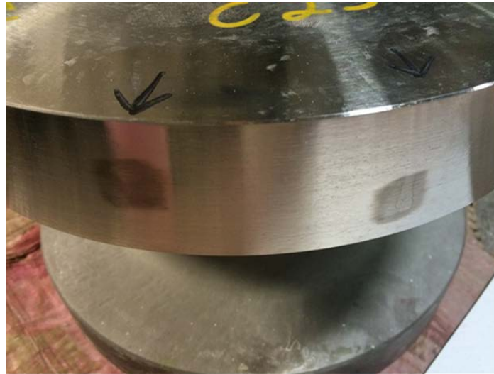
Figure 3-4. Weld Repair of Exhaust Reducer Housing Defect
