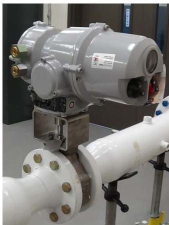
Figure 3-14. Rotork Four Inch Diameter Back-Pressure Control Valve
