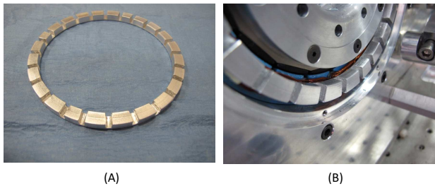
Figure 11. PHOTOGRAPHS OF THE FLEXIBLE ALUMINUM INSERT (A) AND THE INSERT MOUNTED ON THE STATOR COILS (B).
