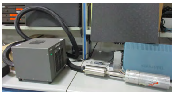
Fig. 35: HPGe Detection System Measurement Setup
