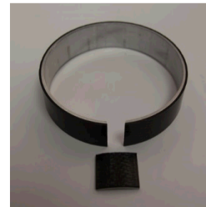
Ring closes in on itself at room temperature due to residual stresses
