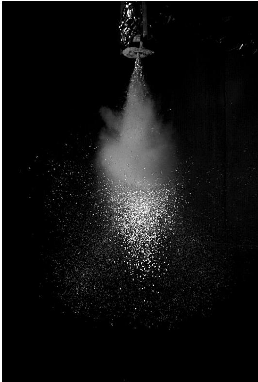
Fig. 2. T3 sodium spray fire during the first couple of seconds.
