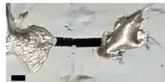
Large Overlap CNT p-n junction film
