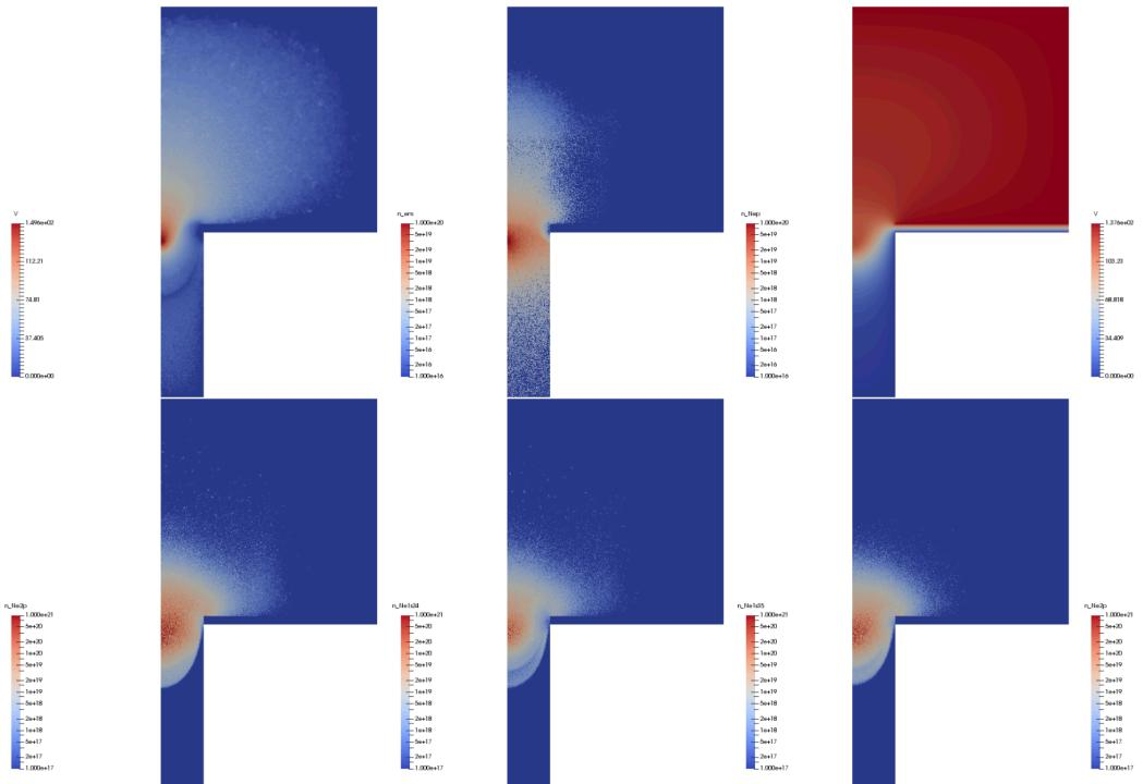
$e^-$  and  $Ne^+$  scales are  $[10^{16}, 10^{18}]/\text{m}^3$ , excited states are  $[10^{17}, 10^{21}]/\text{m}^3$ ,  $V_{max} \sim 140$  V
