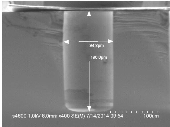
Experiment uses 1-4 cylindrical 50  $\mu\text{m}$  radius cavities (up to 200  $\mu\text{m}$  deep) all connected to the same ballast resistor-in-series circuit.
