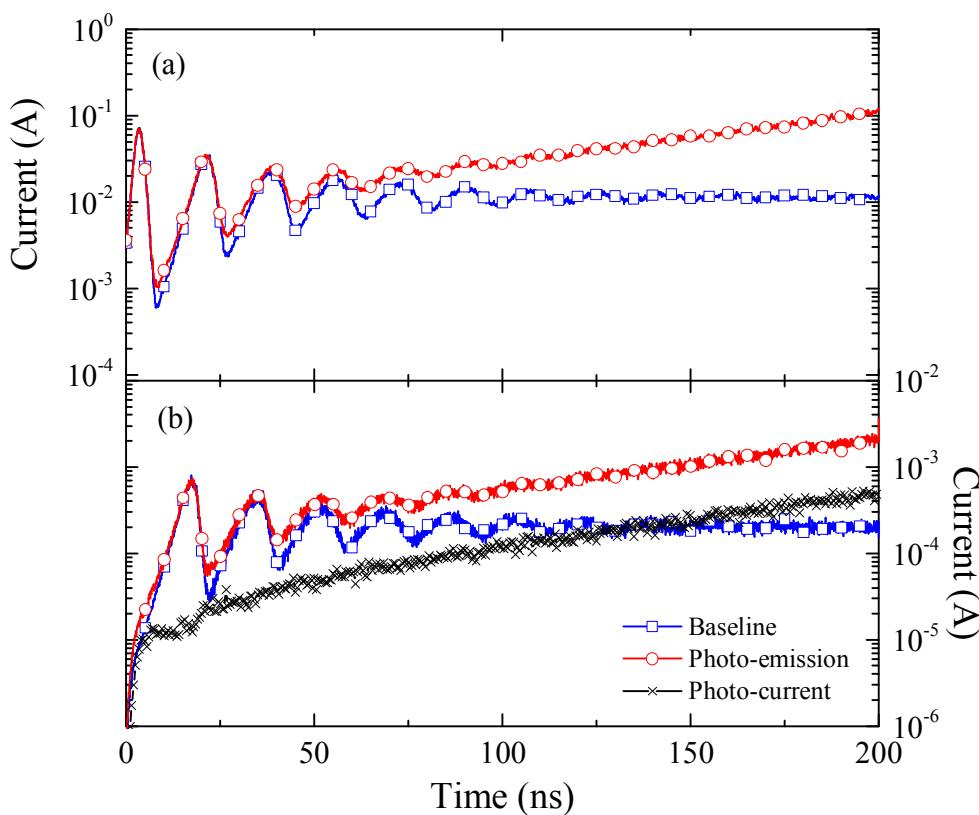
Left: Photo-current accounts for nearly 20% of the total current originating from the cathode as  $t \rightarrow 200$  ns.
