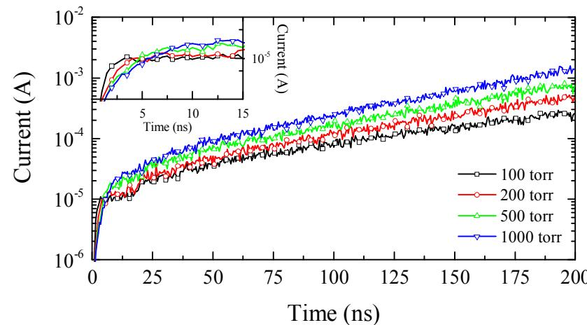
Observed photo-current at various pressures.  $E/n$  was set to result in steady-state without photo-current.
