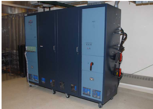
72 V 1000 A Bitrode (2 Channels)
