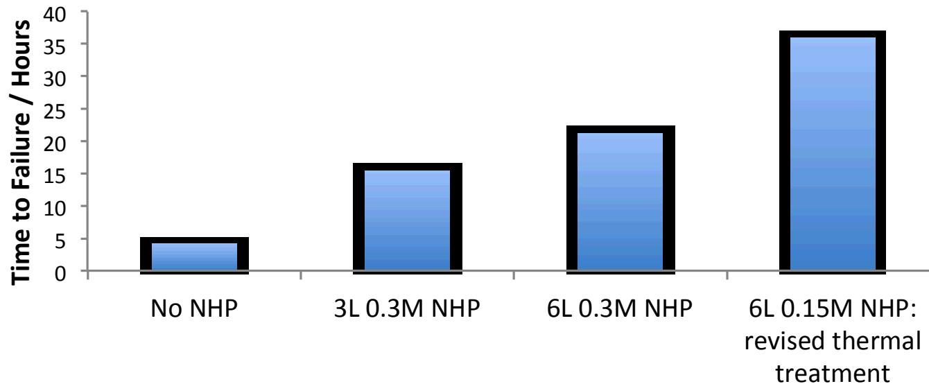
Although thickness and processing conditions of sol-gel film matter, NHP coatings all clearly show improved resistance to alkaline degradation.
