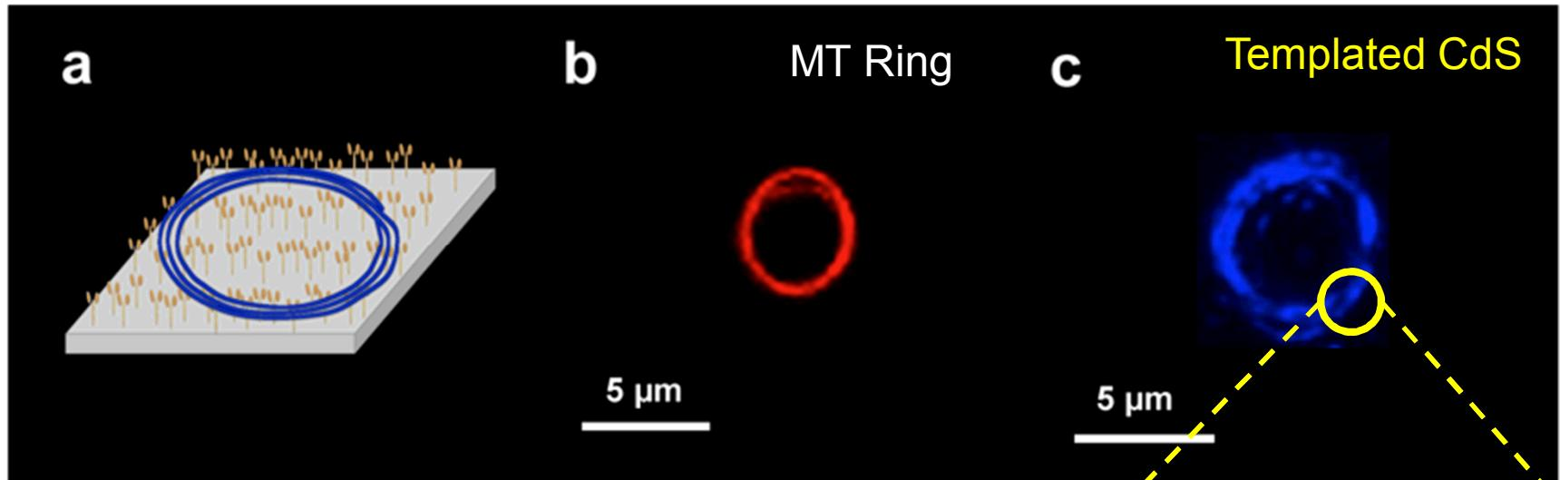
Incubation of MT rings with aqueous  $\text{Cd}(\text{NO}_3)_2$  and thioacetamide leads to controlled templating of CdS nanotube rings.
