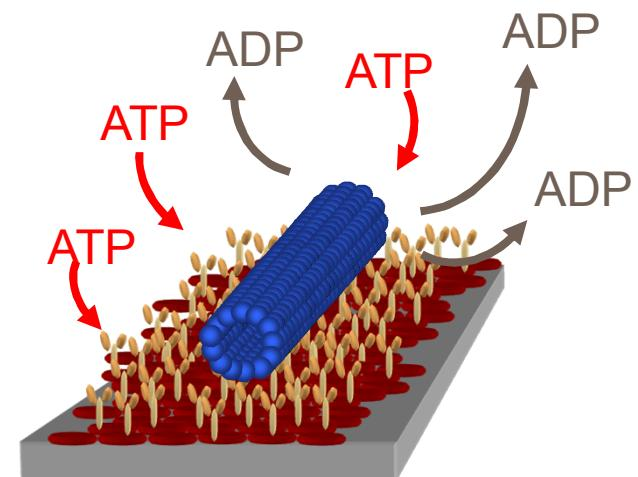
**“Inverted (Gliding) Motility”** relies on array of surface-bound inverted kinesins to capture and transport MTs over a surface.
