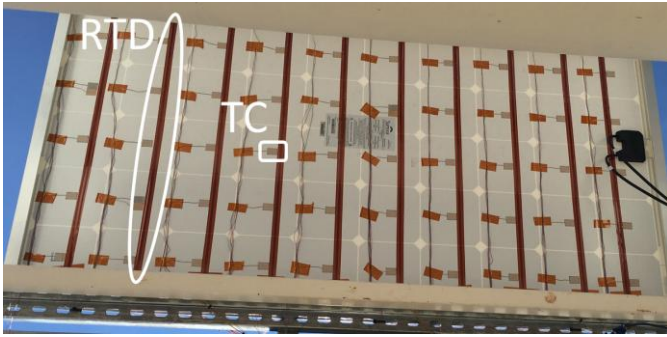
Fig. 2. Module backside with instrumentation
