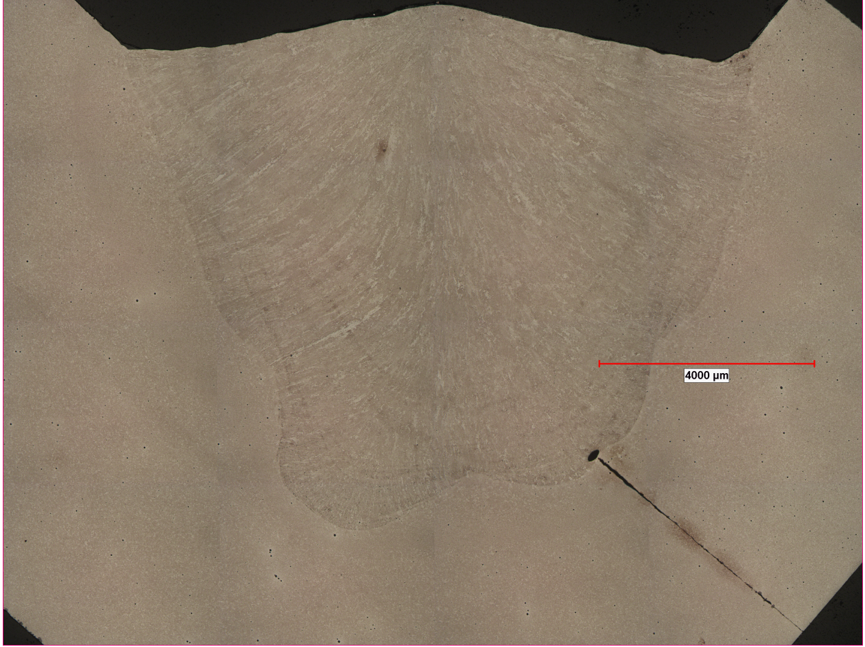
Figure 2: Mosaic image of weld at edge of sample.
