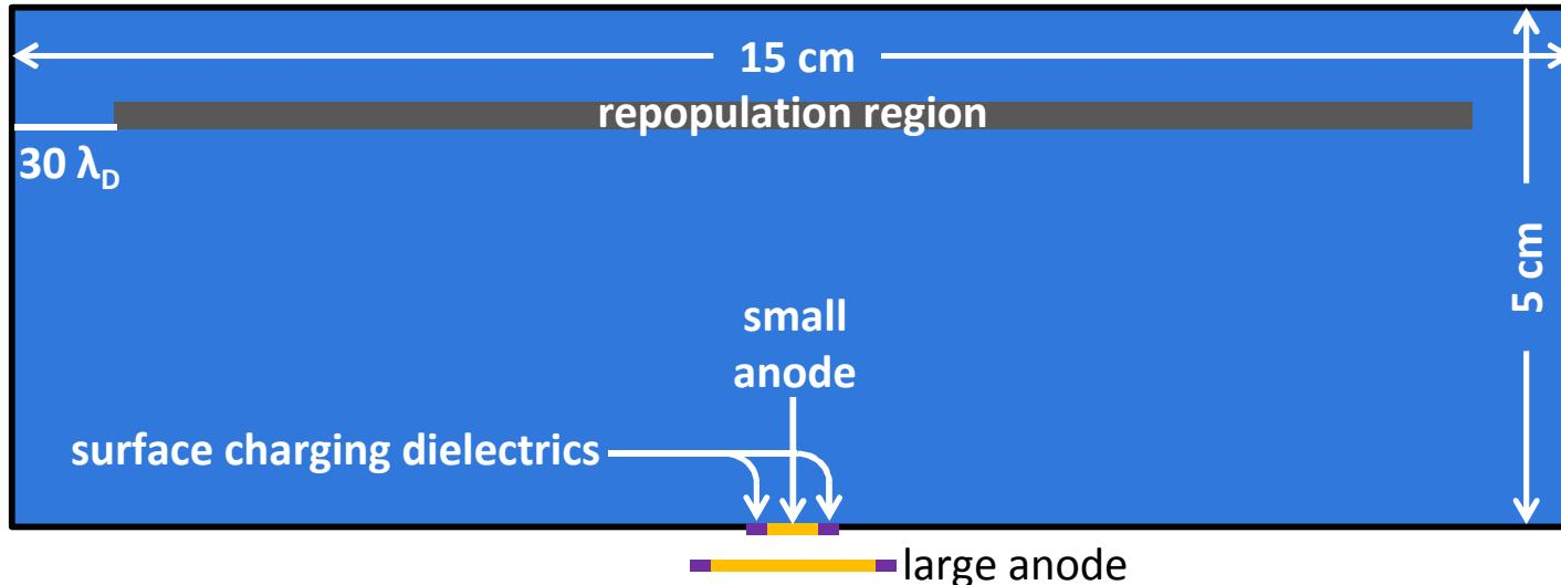
Neutral He plasma is generated in the repopulation region ( $T_e = 4$  eV,  $T_i = 0.1$  eV) at a rate to match experimental densities in the near-anode region,  $n_i = n_e \sim 10^9/\text{cm}^3$  ( $\sim 2 \times 10^9/\text{cm}^3$  in the repopulation region).
