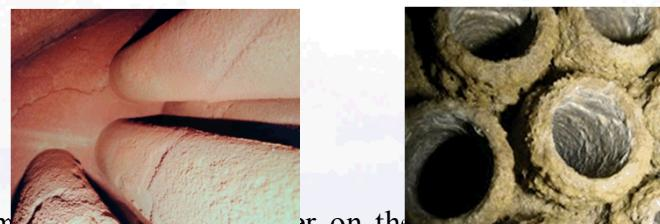
Formation of scale layer on the tube and walls which disrupts the boiler function due to the very low thermal conductivity of the silica scale.<sup>3</sup>
