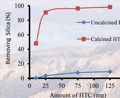
The applied sorbent was tested in two different forms: uncalcined HTC and calcined HTC at 550 °C. This result indicated that the calcined HTC removes greater amounts of silica compared to uncalcined HTC.
