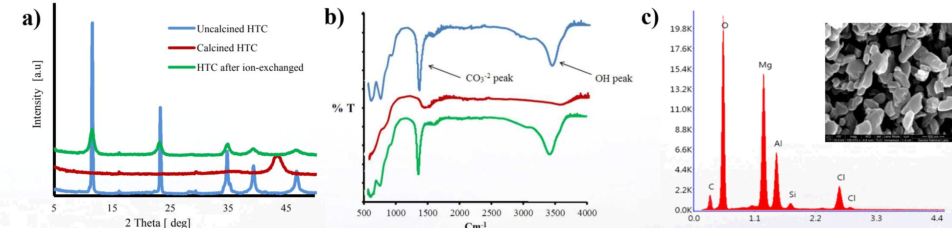
FTIR and XRD analysis support the fact that calcined HTC can be reconstructed to original structure by exposure to the cooling tower water containing silica ions (figures a and b). The presence of silica at HTC structure after reconstruction was confirmed by SEM-EDS spectroscopy (figure c).
