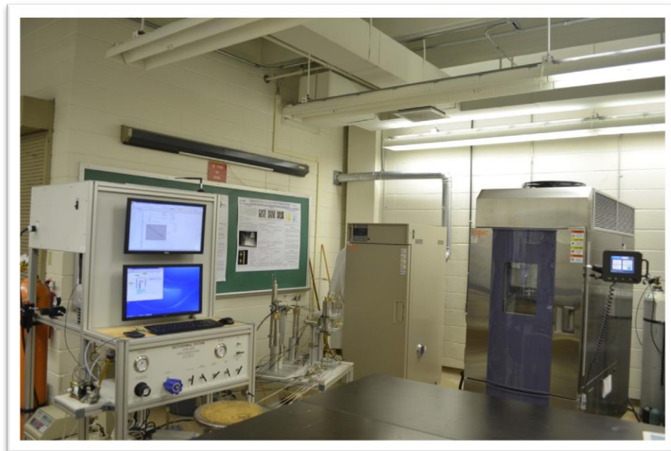
Figure 35: From Left to right, Liquid Pressure-Pulse Decay Permeameter, Vertical Temperature Chamber, and Temperature Cycling/Relative Humidity Chamber respectively.
