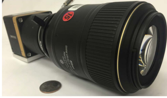
Figure 6. The plenoptic camera used for the results reported here [7].
