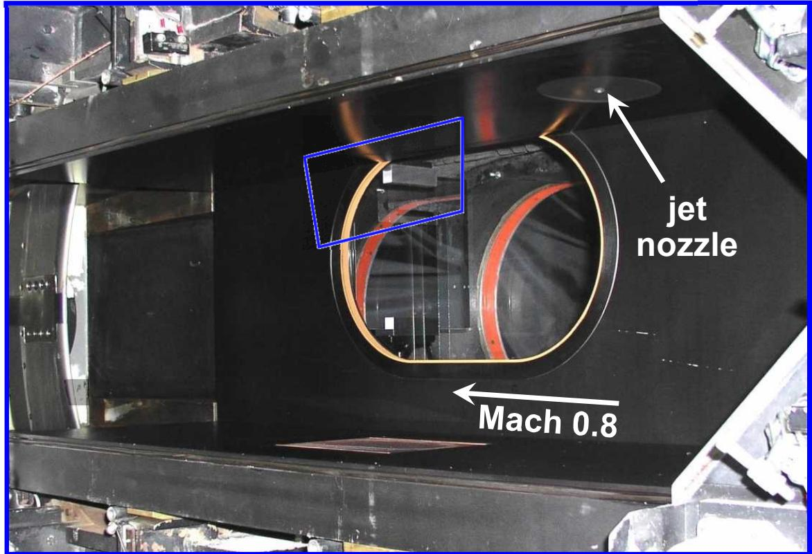
A jet nozzle mounts on top wall of TWT, driven by high-pressure air.
