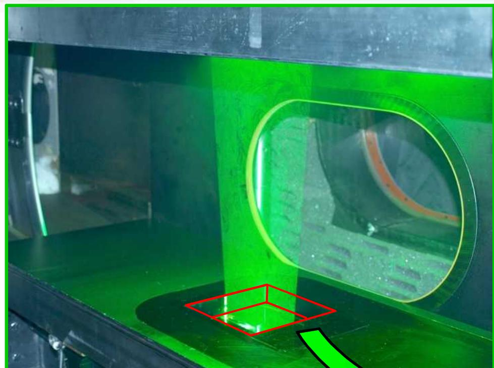
Our cavity is a rectangular cutout built into the test section floor:
