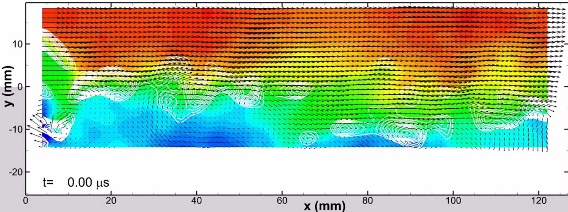
The pulse-burst PIV field of view visualizes most of the recirculation region including reverse velocities.
