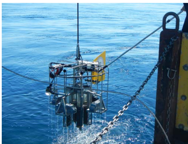
Figure A4. Mini-multicoring rig provided by UCLA for the R/V Sharp cruise being retrieved off the port stern of the ship. The fiberoptic cable available at this location on the ship was used to provide real-time video feeds from the seafloor using a camera system built by USGS engineer G. Hatcher. See Hatcher et al., 2015.
