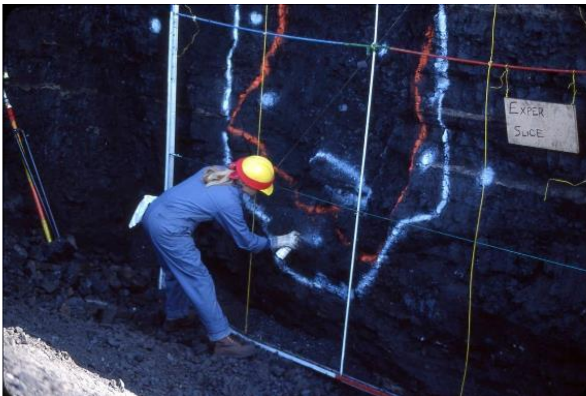
Figure 15. All five of the Centralia Large Block tests were excavated, inspected, described, and documented. This advanced an understanding of the rubble-filled nature of UCG cavities. (LLNL photo)
