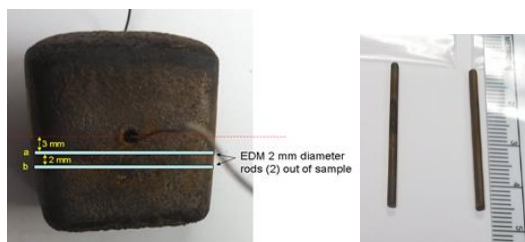
Figure 36. A typical ATAS cup cast sample. Lines show where the rod samples were machined for evaluation.
