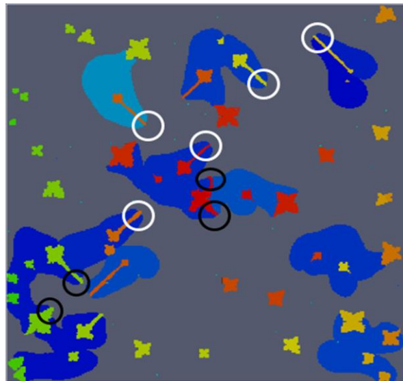
Figure 57 Cooperative growth of flake-like graphite precipitates with same austenite grain on both sides (white circles) or with two different austenite grains (black circles); austenite grains are represented in shades of blue color, graphite is red, and liquid phase is gray
