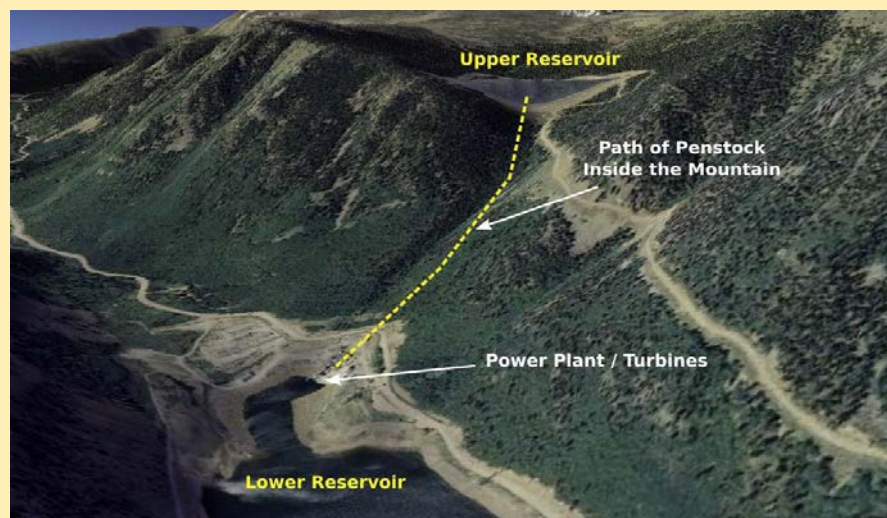
Figure 1. Arrangement of power plant, reservoirs, and penstock pathway.
