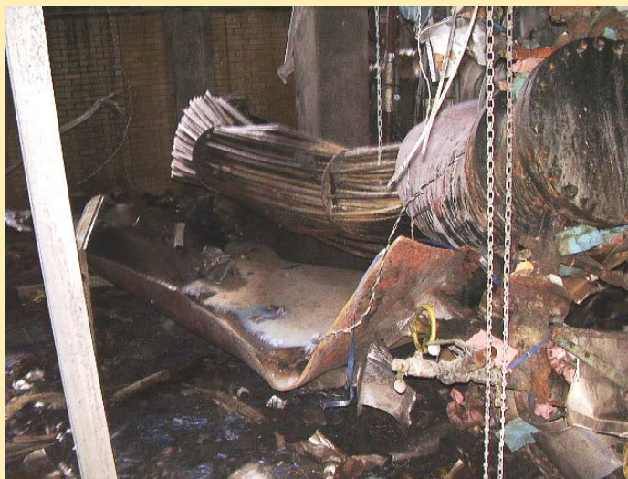
Above: Debris resulting from heat exchanger rupture and ammonia release.
