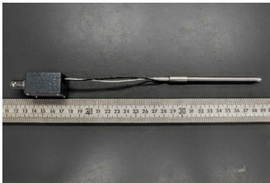
Figure 5.4: Helium-3 proportional counter [6].
