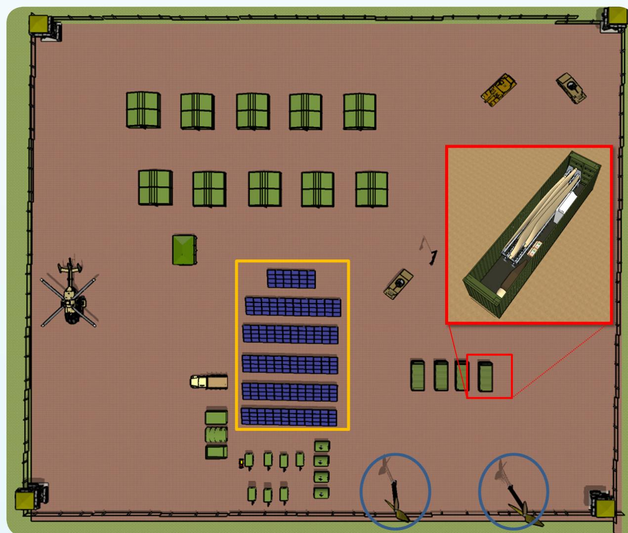
A sample installation of renewables at a 200-soldier contingency base with diesel generator sets. Here 60 kW of wind energy and 85kW of solar are added to 210 kW of diesel generators. Energy sources differ additionally in their land use and required transport.
