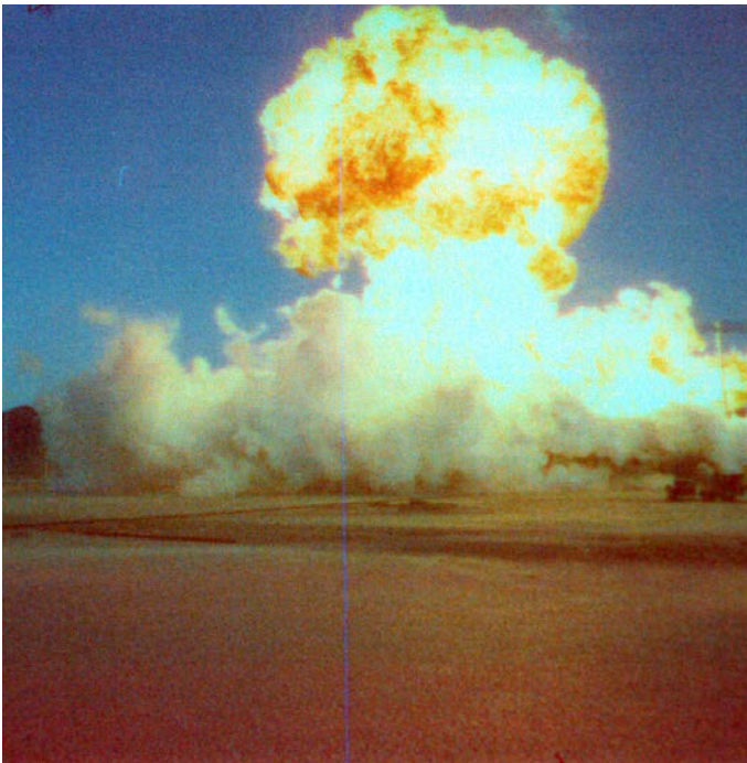
Fireball from accidental ignition of Falcon5 LNG test in 1987 1
