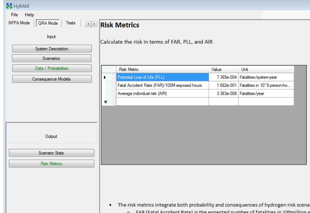
The screenshot shows the HyRAM software interface. The top menu bar includes File, Help, NFPA Mode, QRA Mode (which is selected), Tests, and a navigation bar with back, forward, and search icons. The left sidebar has tabs for Input (System Description, Scenarios, Data / Probabilities, Consequence Models) and Output (Scenario Stats, Risk Metrics). The main right panel is titled 'Risk Metrics' and contains the following table:
