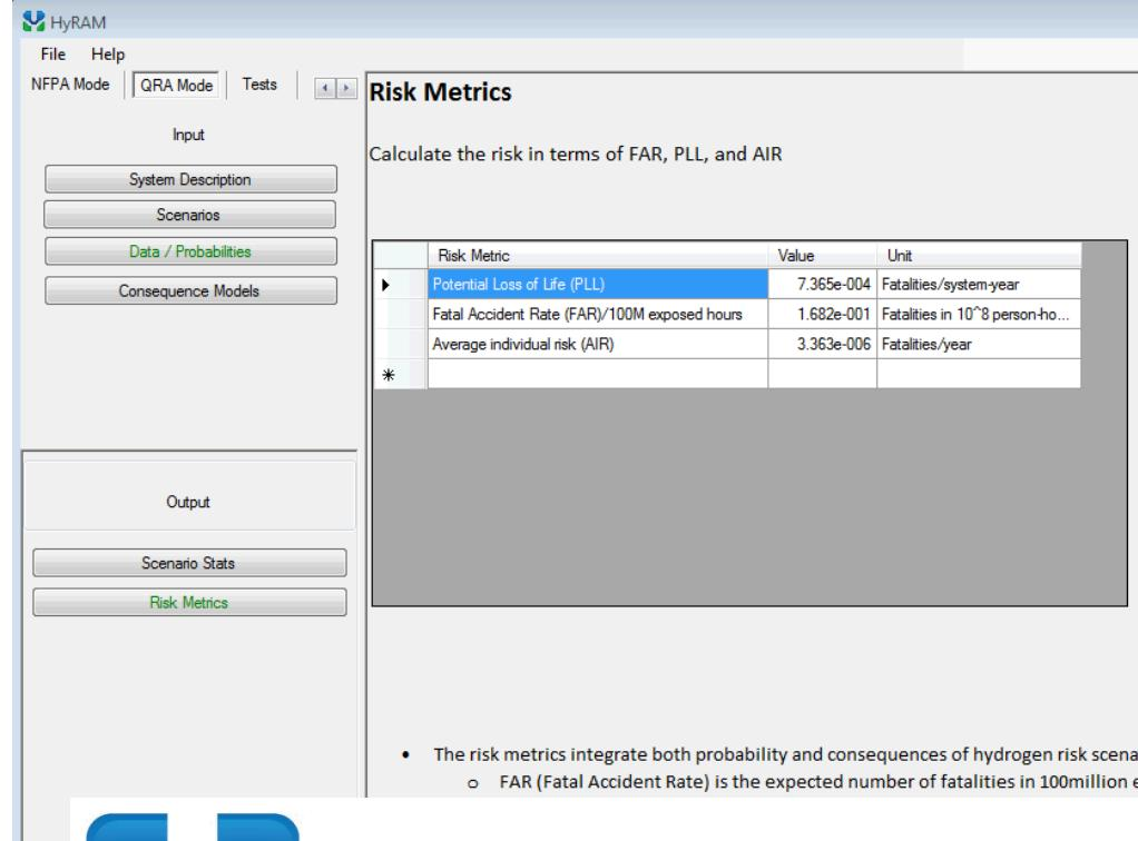
The screenshot shows the HyRAM software interface. The top menu bar includes File, Help, NFPA Mode, QRA Mode (which is selected), Tests, and a toolbar. The left sidebar under the Input tab shows buttons for System Description, Scenarios, Data / Probabilities (which is selected), and Consequence Models. The right panel is titled 'Risk Metrics' and contains the following table:
