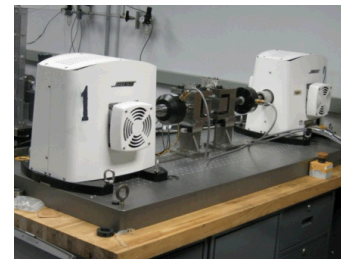
Used fuel rod stiffness Experiments (in hot cell and out) and analyses of stress distribution
