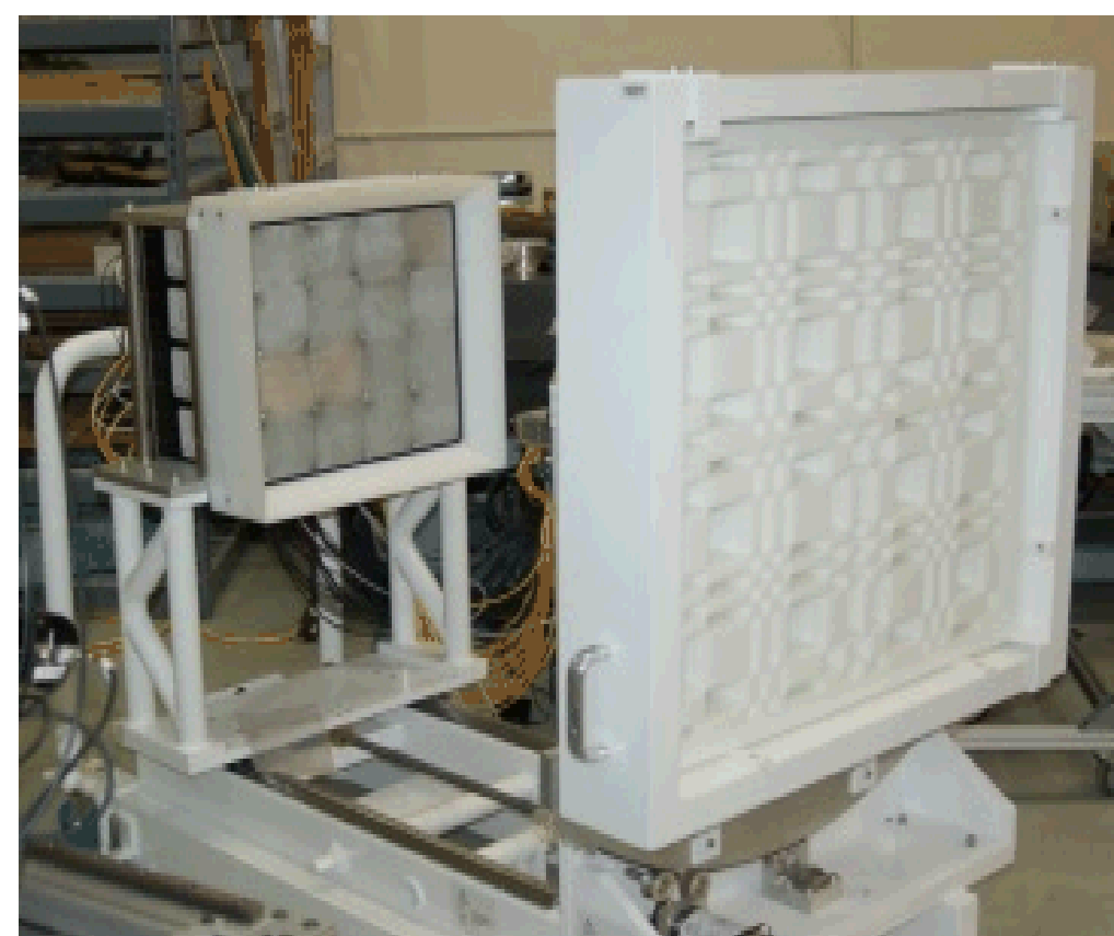
Figure 2 Fast-Neutron Coded-Aperture Detector
