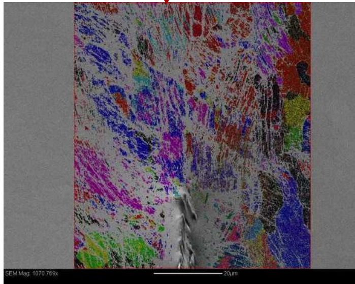
EBSD inverse pole figure map near crack tip
