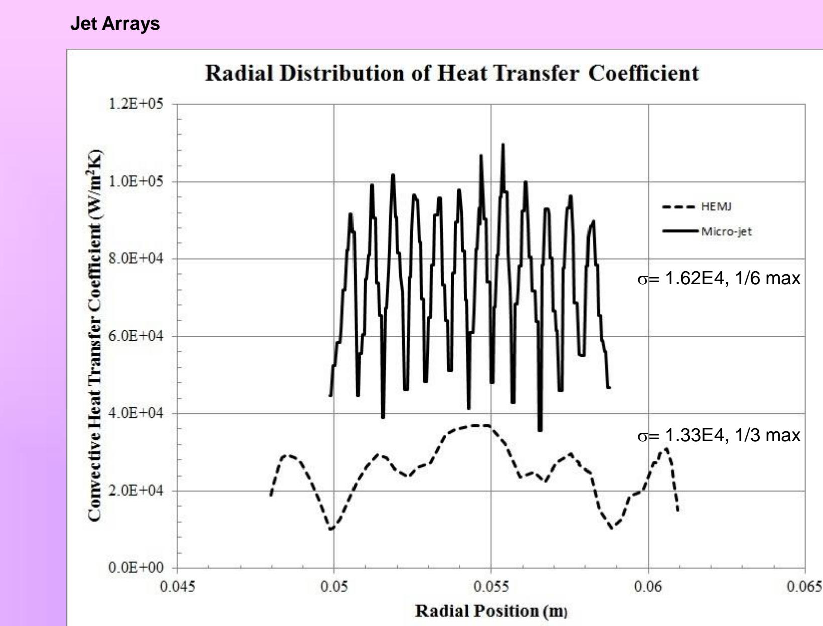
Both the HEMJ and the micro-jet array performed well under spatially non-uniform heating. No evidence of flow instabilities appeared in the simulations. Although the density and velocity distributions in the exit plenum changed significantly due to the heating, no appreciable difference in the mass flow distribution resulted under the heated wall or through the jet array.
