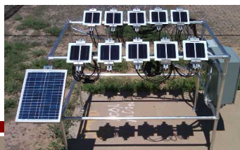
Soiling station being built at ASU
