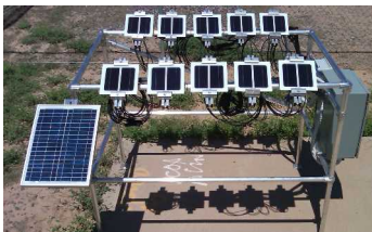
Soiling station being built at ASU
