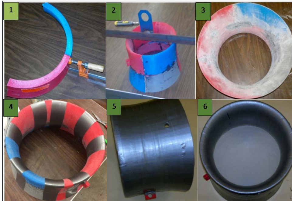
Figure 27. Experimental shroud (Shroud manufacturing steps): (1-2) glued parts together (3) sand the surfaces to be smooth (4) taped the whole model (5-6) complete model
