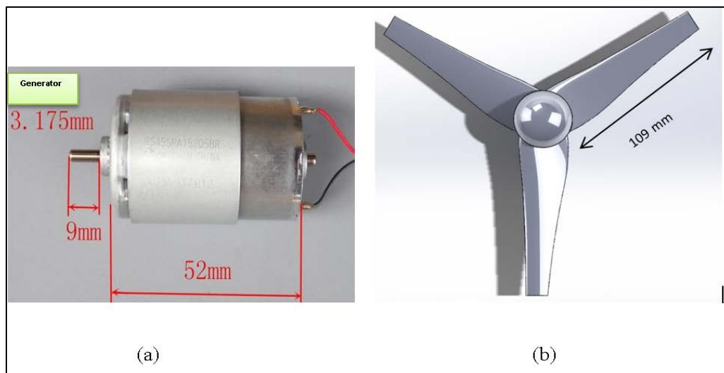
Figure 29. Micro-wind turbine: (a) Micro Generator (b) Airfoil NACA4415 and Nacelle
