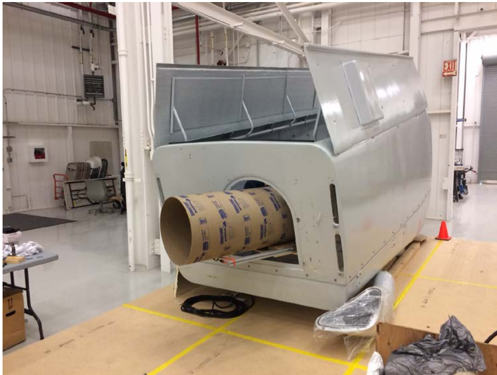
Figure 31. Lidar mount mock-up with 20-inch diameter sonotube to represent the lidar installed in WTGa2 nacelle at Sandia.
