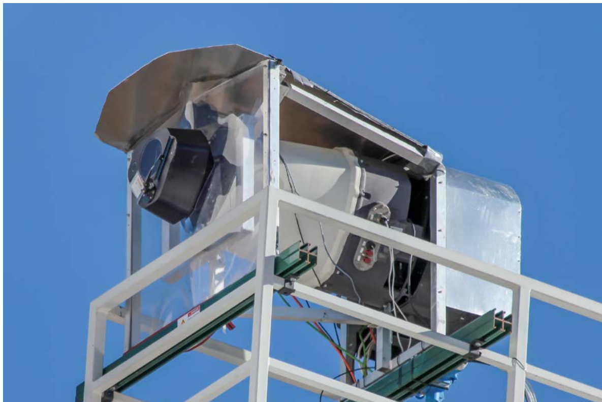
Figure 34. Mounting system of DTU SpinnerLidar at NREL showing the front and rear covers
