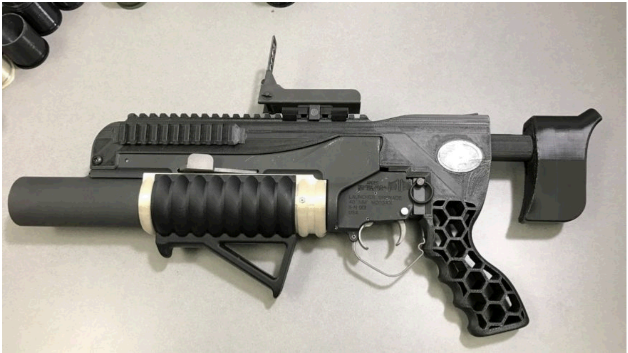
Figure 27. An example of a working system using AM manufacturing: US Army grenade launcher [Hodgkins, 2017].
