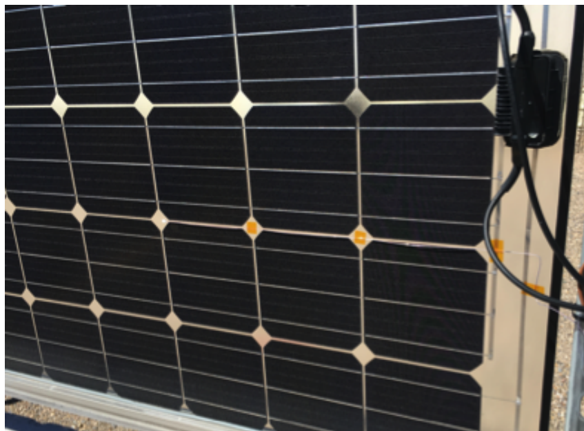
Figure 2: Backside of Prism module showing location of yellow thermocouples.
