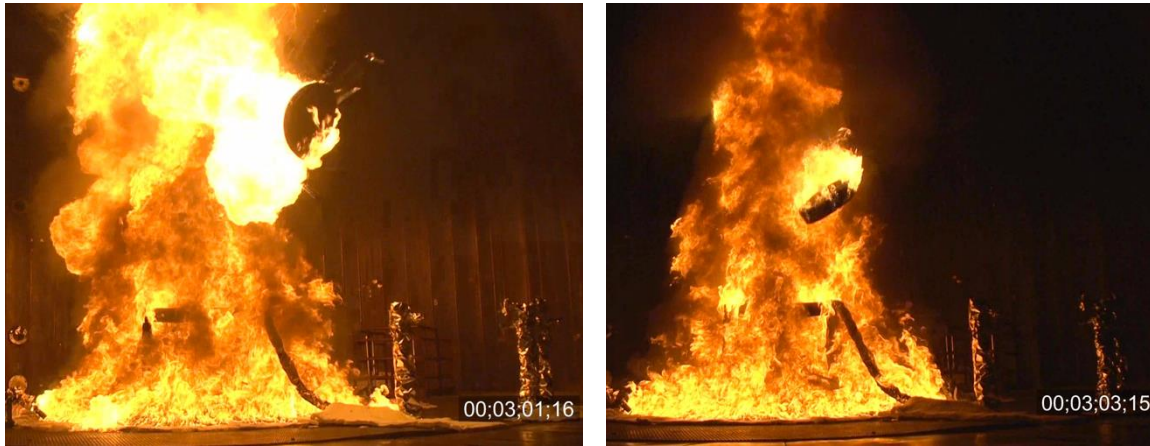
Figure 56. Videos screen captures of Phase II Test # 1 showing ejection of lid.
