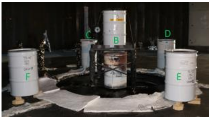
Figure 59. Image of the test layout in Test #2 of Phase II taken from the southeast corner of the facility.
