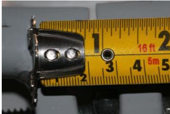
Figure 11. Gap that remains in the drum ring after torquing to 60 ft-lb. Image taken from the first test in phase II.
