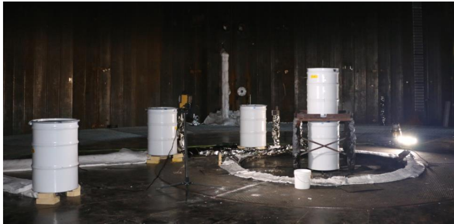
Figure 3. Typical fuel-pool/drum layout inside of FLAME.
