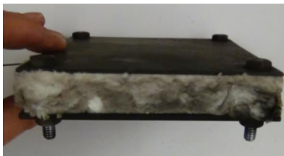
Figure 9. Heat Flux Gauge (HFG) used in POC and 7A fire tests.
