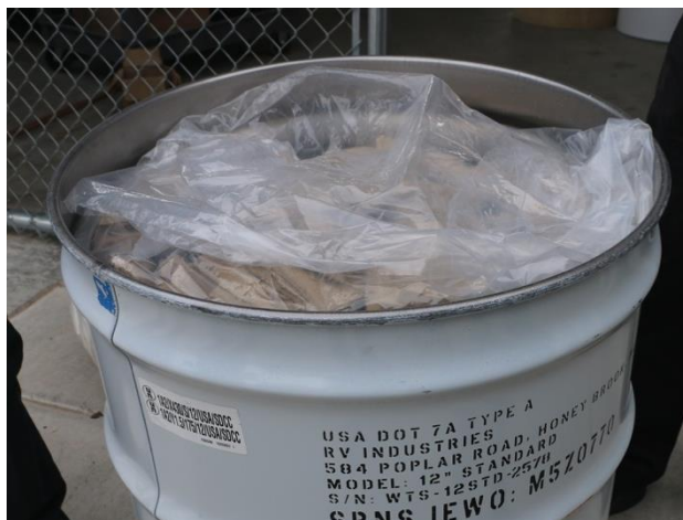
Figure 7. Drums outside the fire filled with chipped Celotex.
