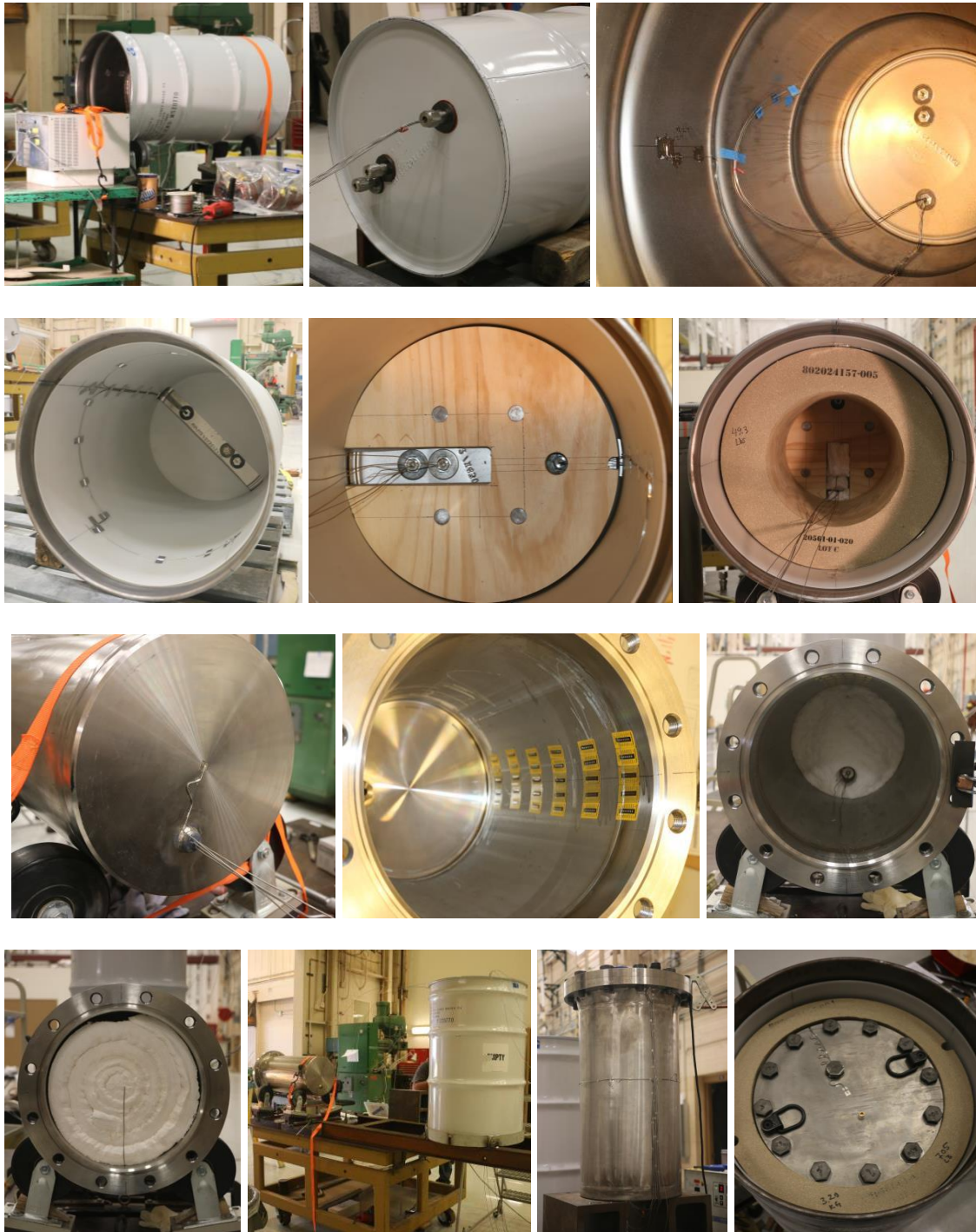
Figure 8. Series of images showing the process of instrumenting and assembling POCs in preparation for Phase I test. Images are from the first test.
