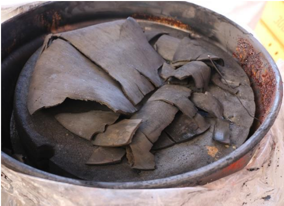
Figure 18. Internal remains of POC after Test #1: (a) drum A and (b) drum B with and without the PC.
