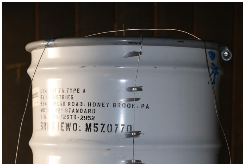
Figure 13. Sacrificial TCs routed through the top of the POC to detect the time when the lid popped open or was ejected.
