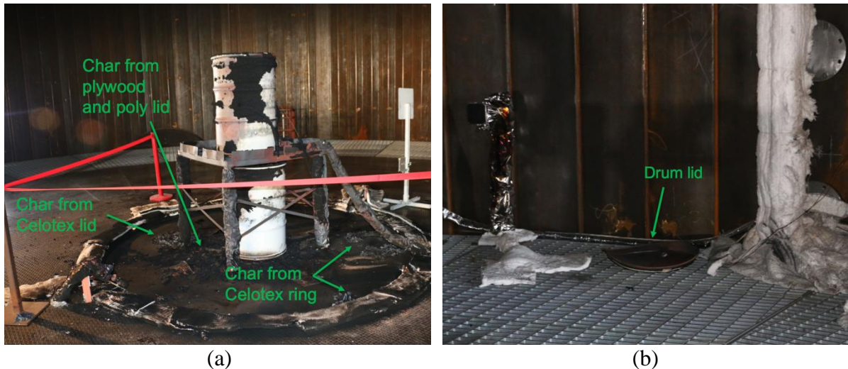
Figure 57. Test remains after Test #1 in Phase II. (a) center of the pool and (b) lid by the wall of the test cell.
