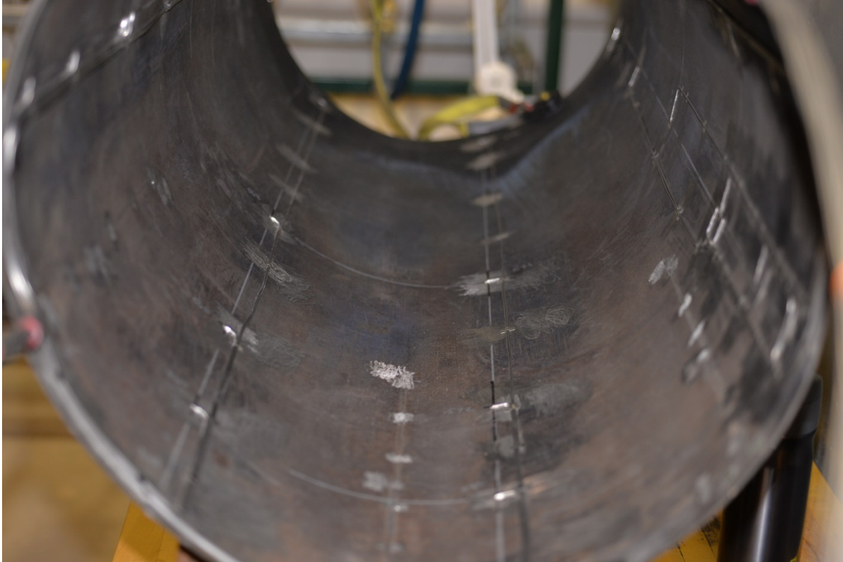
Figure 6. Inside Surface of Shroud with TCs Installed.
