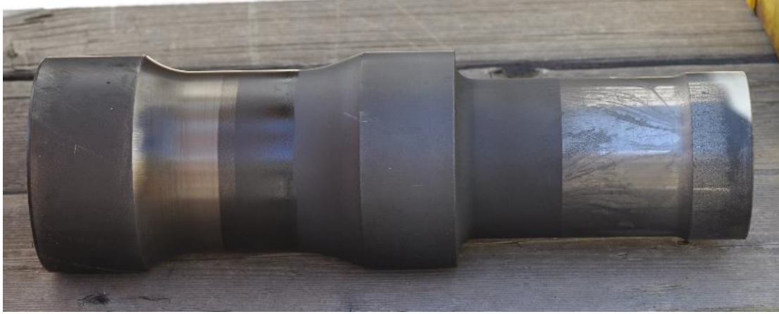
Figure 25. Piston with no lubrication at 400°F
