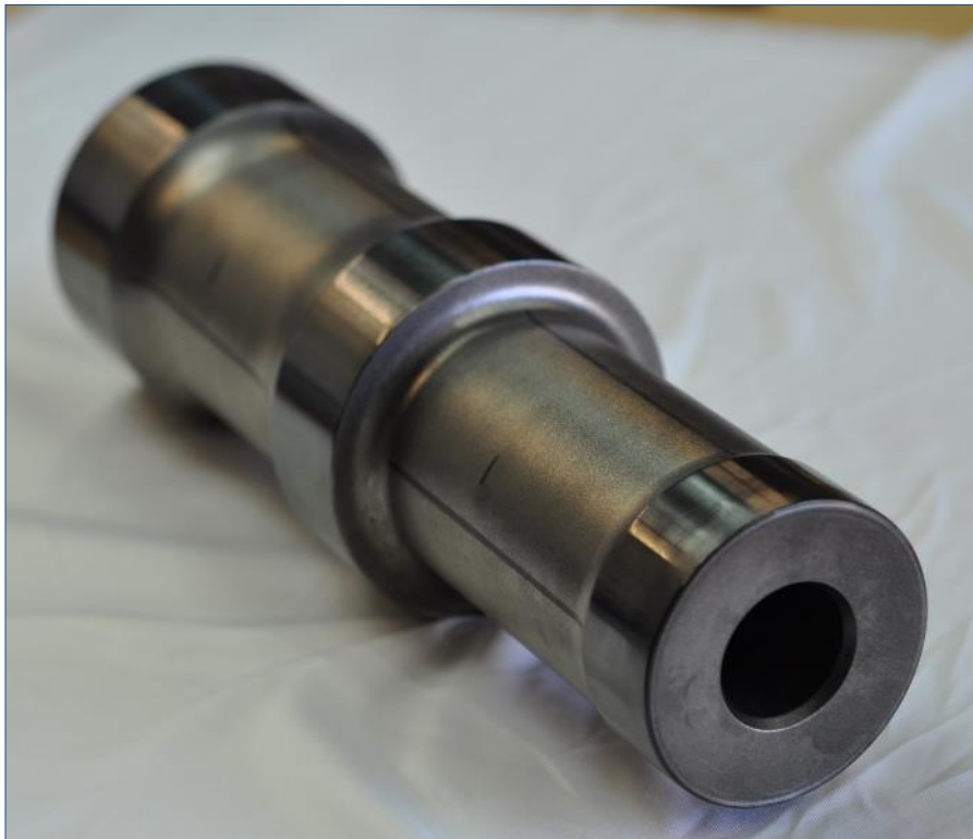
Figure 35. LT piston with DLC coating applied
