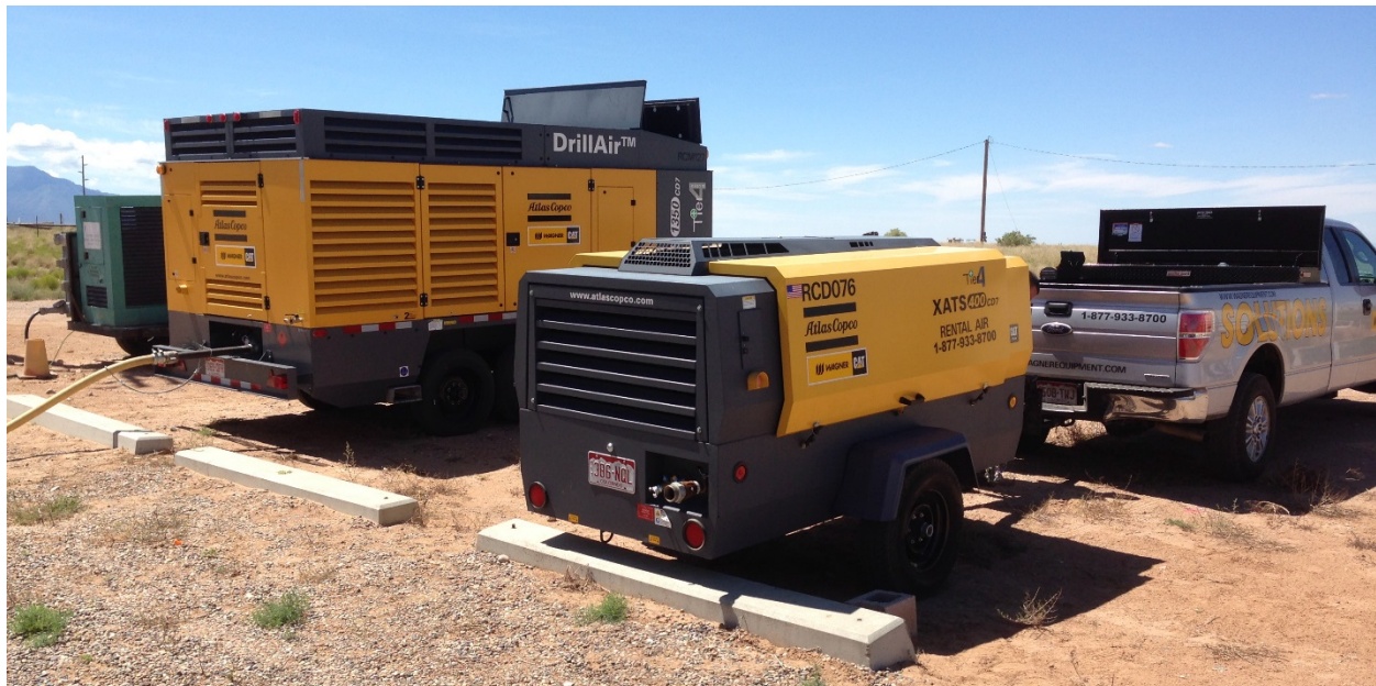
Figure 62. High-pressure compressor for AC-500 sub-system and low-pressure compressor for MOTOR-150
