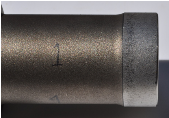
Figure 31. HT piston wear progression (stem end)
