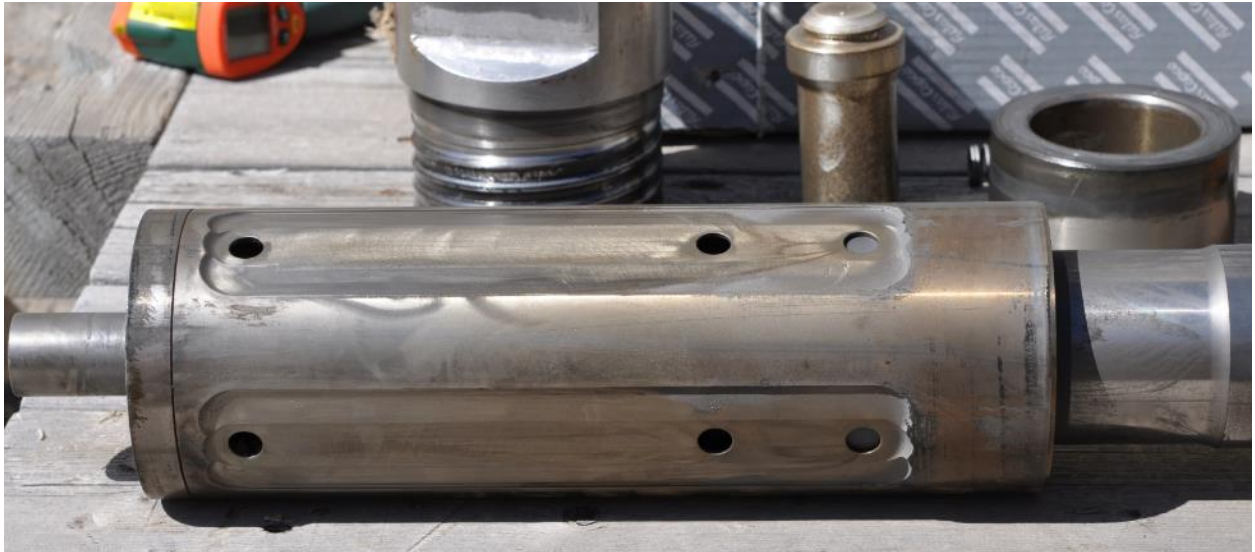
Figure 23. Piston sleeve assembly after operating at 400°F
