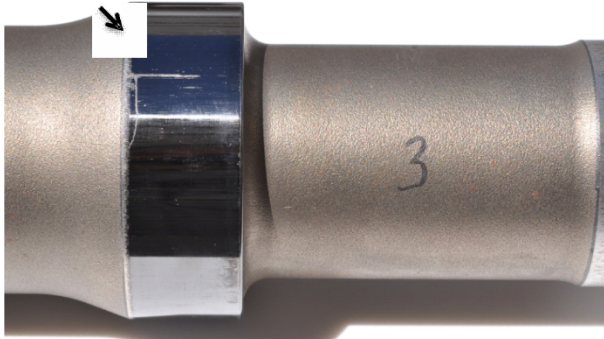
Figure 32. HT piston wear progression (mid-section)
