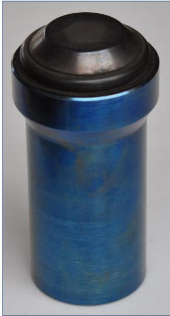
Figure 47. Check valve tempering temperature color change
