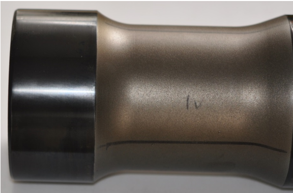
Figure 41. LT piston visual wear after 25.5 ft
