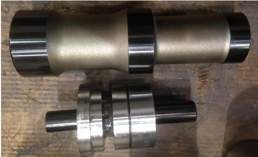
Figure 16. High-temperature prototype after first run
