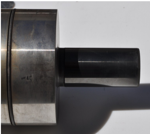
Figure 34. HT distributor wear progression
