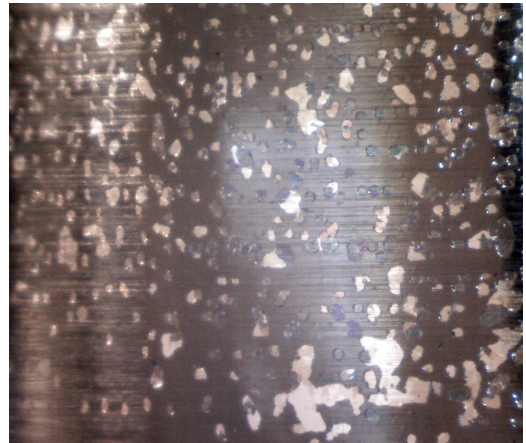
Close-up view of "pits" on distributor surface(50x zoom)
