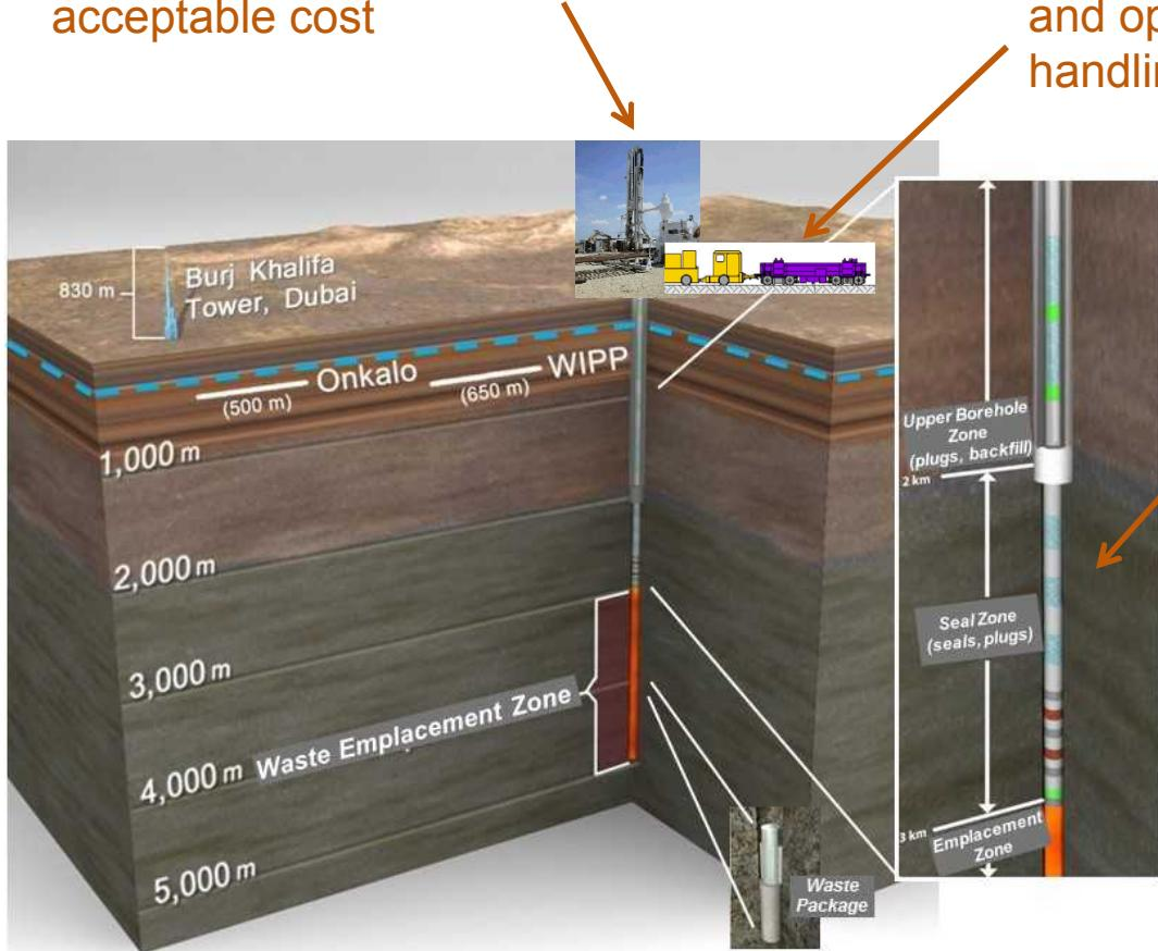
Waste package emplacement system can be engineered to maintain structural integrity and operational safety during surface handling and downhole emplacement
