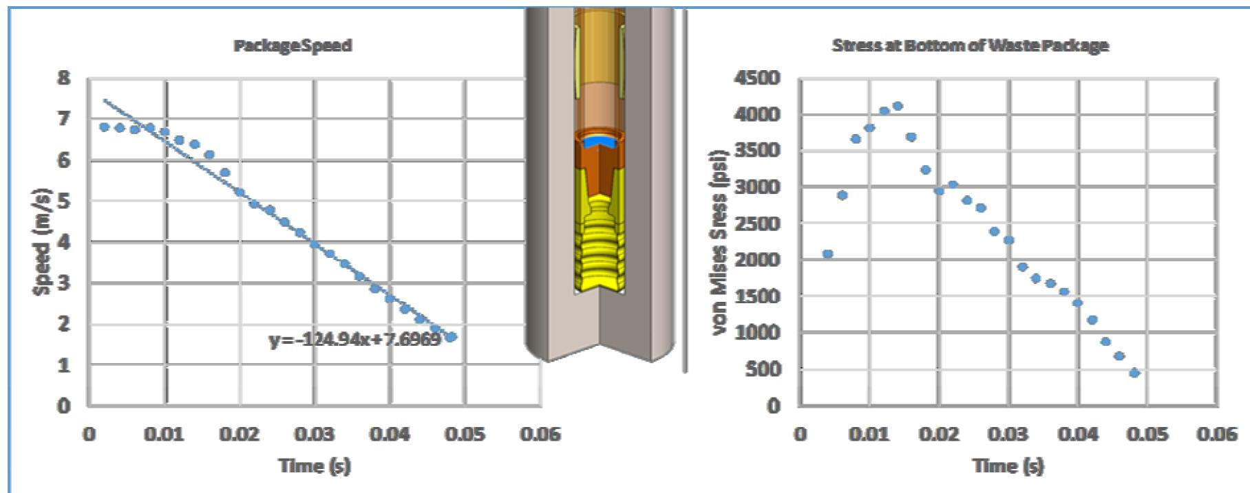
Simulation results for vertical end-drop from 3 m onto compacted gravel.
