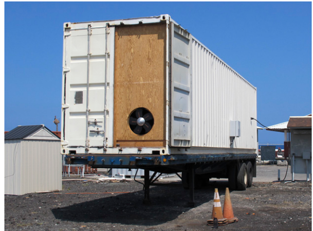
FIG. 5. Rotary subwoofer of the Infrasound Laboratory of the University of Hawai'i at Mānoa.
