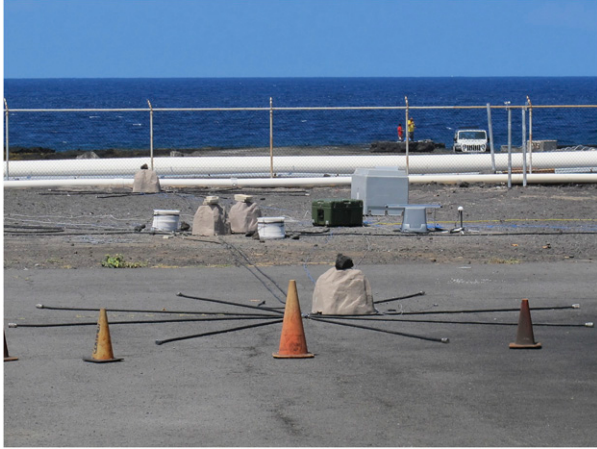
FIG. 6. Overview of the experiment setup. The pipe array is laid on the ground. Sensors and digitizers are covered by plastic boxes. The plastic boxes near the center of the array include power and communication system equipment.
