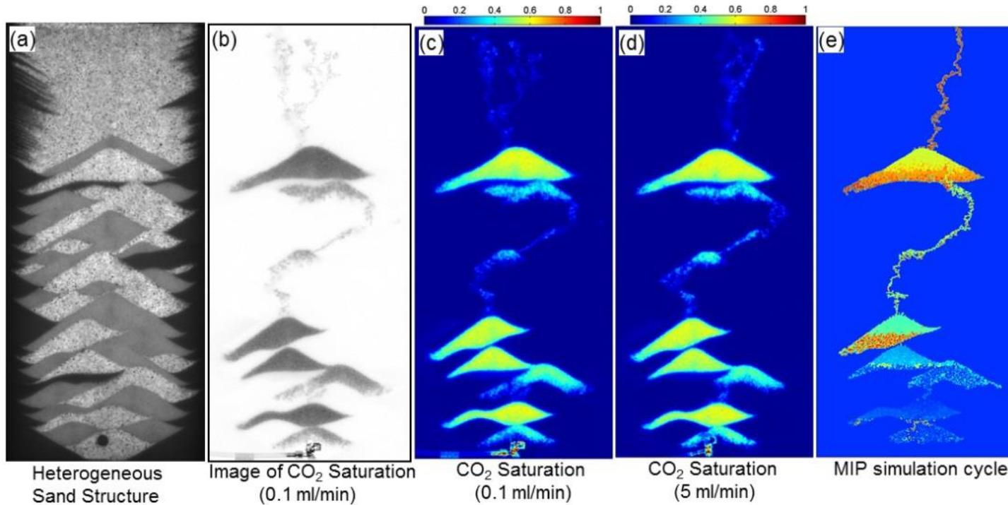
(a) Experimental heterogeneous sand structure (26 cm wide, 55.5 cm tall) of Glass et al. showing the fine sand (dark, #50-70), medium sand (gray, #30-40), and coarse sand (light, 12-20) units.
