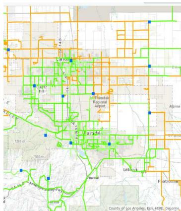
Assign hosting capacity values to the rest of the feeders in each cluster to create a hosting capacity map for service territory
