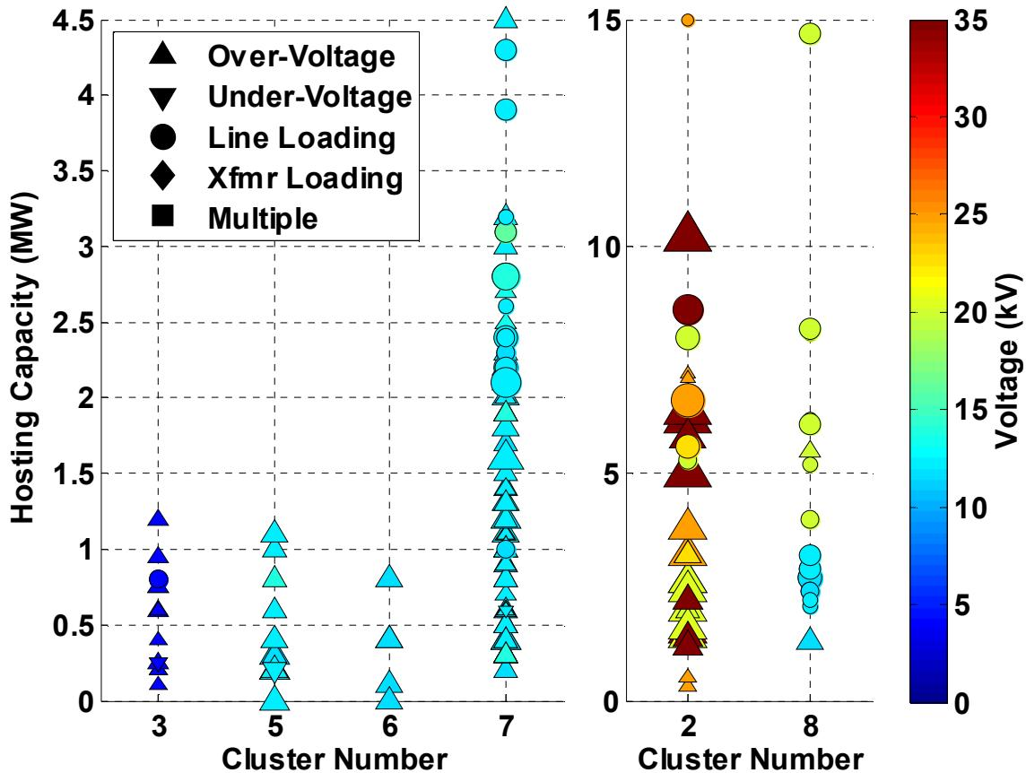
Hosting capacity violation type shown by marker shape for each feeder in the same 6 clusters.
