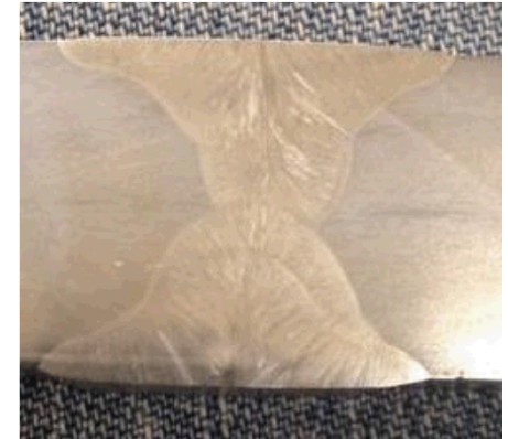
Weld zone, 304 SS plate. Photo: Ranor
