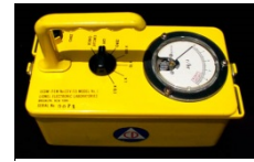
Figure 29: The CDV-715 has a range of 0-500 mR/h on its most sensitive scale.
